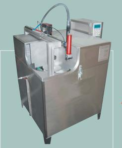
type W 80 as special version for high pressure use, rinsing with demineralized water by ion-exchanger, drying with hot air
